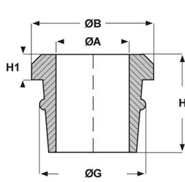
**BOCCOLE PASSACAVO IN PLASTICA CON NERVATURA**
